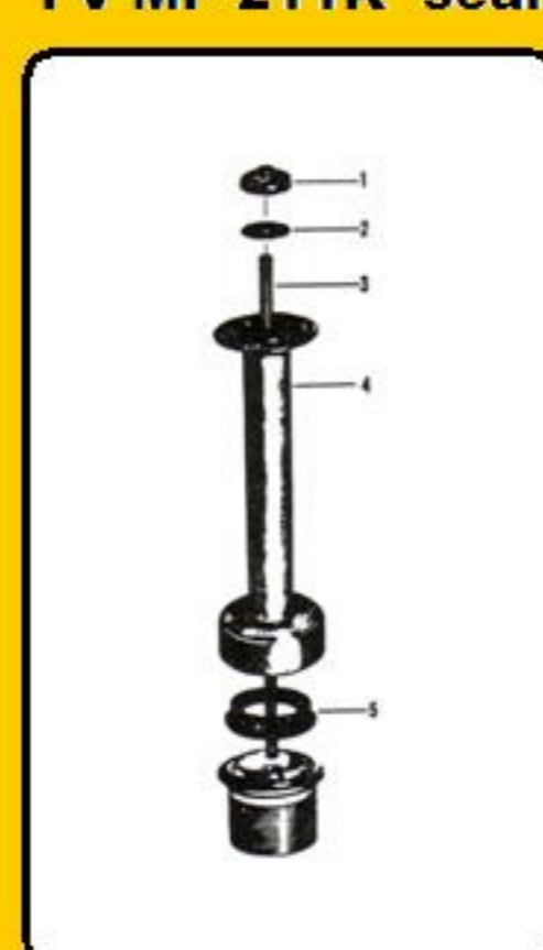
American Standard Flush Valve FV AS 55K parts 1, 2 and 5 FV AS 55S feather washer part #5
